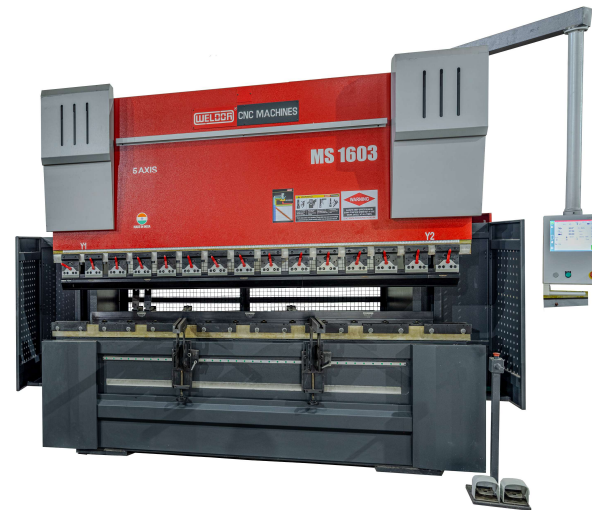
MS SERIES CNC HYDRAULIC PRESS BRAKE WITH MAIN MOTOR SERVO
